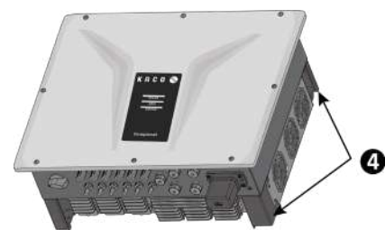
Fig. 7. Lift the unit
