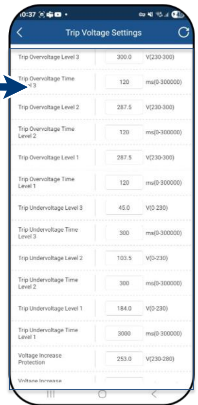
Fig. 119. Define voltage range and shutdown times
