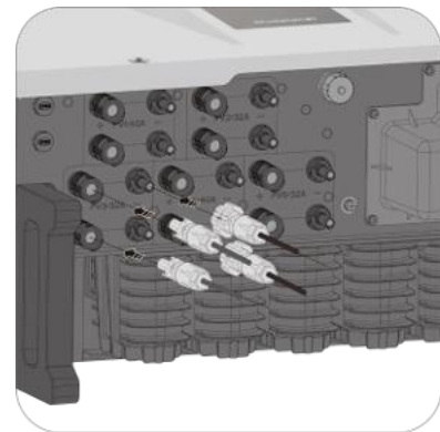
Fig. 27. Current-carrying capacity and plug in PV connector
