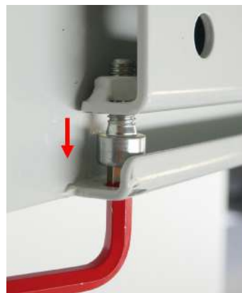
Fig. 17 Bracing the storage unit
