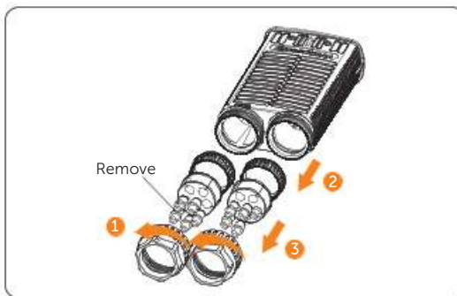
Figure 7-9 Disassembling the AC connector
