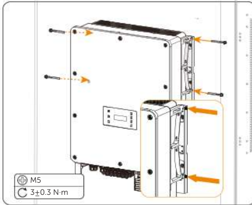
Figure 6-28 Securing the inverter
