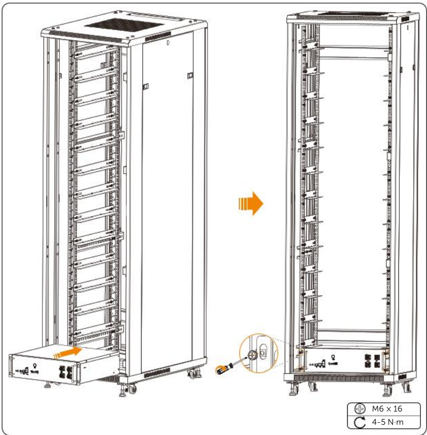
Figure 6-18 Placing battery modules and tightening M6 screws
