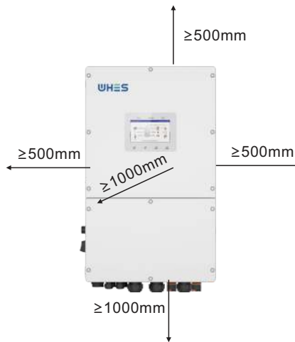
Figure 3.5 Inverter Mounting Clearances
