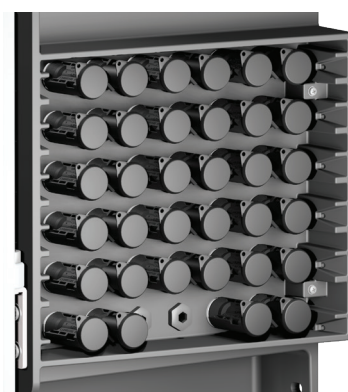
M100A: 8 MPP trackers for 2 module strings each
