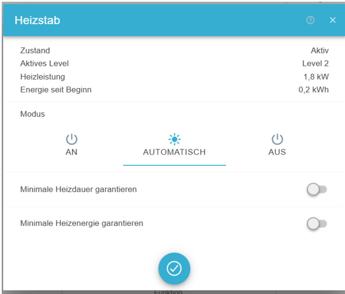
Figure 12. Heating element — "Automatic" operating mode
