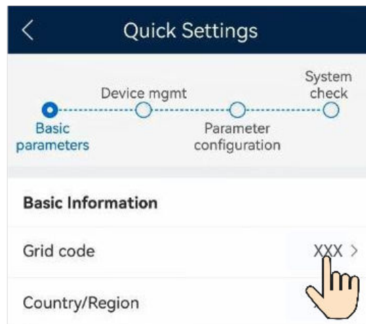
Figure 4-16 Setting the grid code (Island-Grid) for off-grid operation
