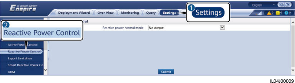
Figure 6-49 Reactive power control
