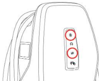
Fig. 13: Activate access point (example)
