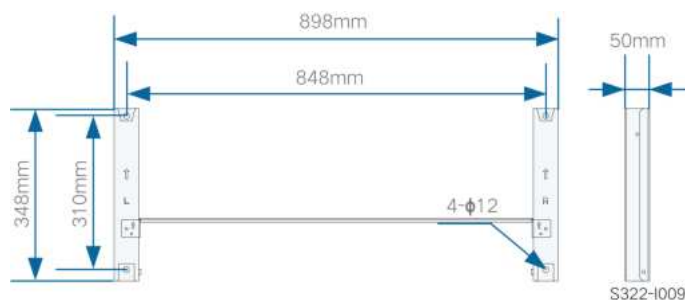
figure 4-1 Dimensions of Mounting-bracket
