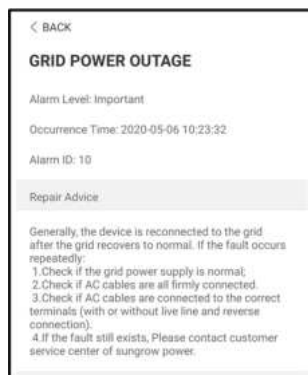
figure 7-9 Detailed Fault Alarm Information
