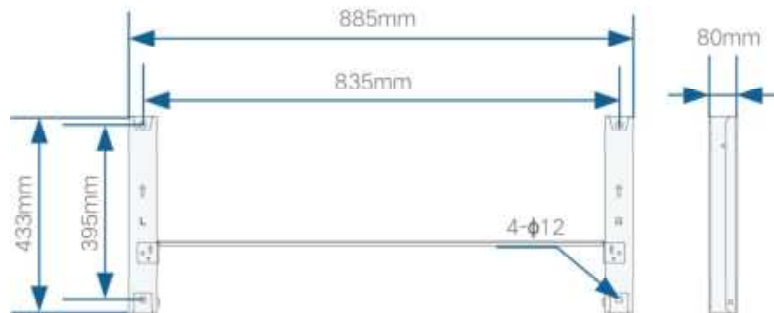
Figure 6-1 Dimensions of Mounting Bracket
