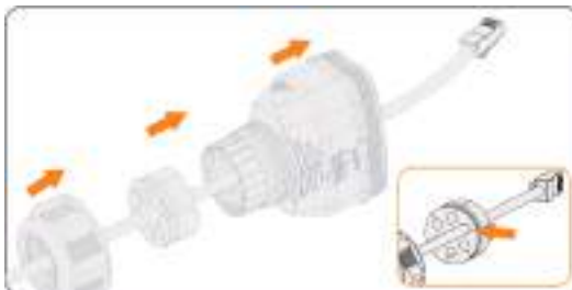
Figure 8-44 Threading the cables
