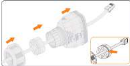
Figure 8-54 Threading the cables
