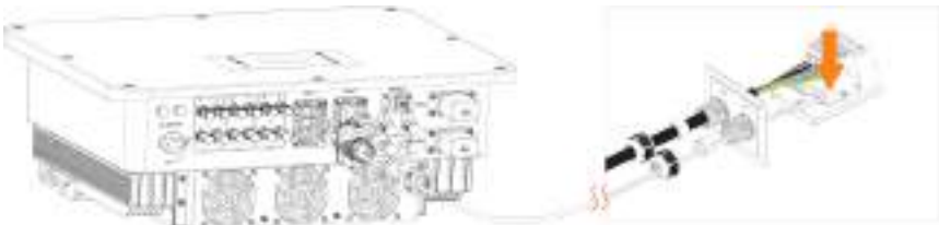
Figure 15-9 Connecting to EV-Charger
