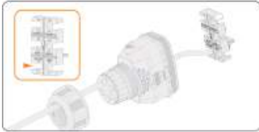
Figure 8-45 Installing RJ45 terminal to the cable fixture
